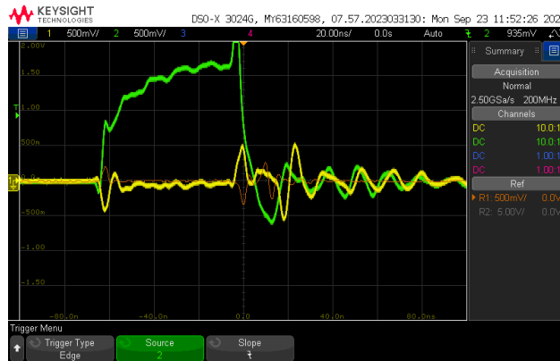
Figure 8: Switching Noise with Separate Return Path
